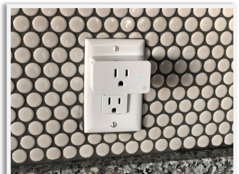
Smart plugs can cut power (or return power) to non-smart devices, like coffee makers, phone chargers and other items that draw phantom load.
